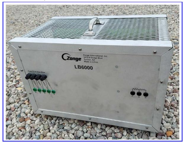
The LB6000 is a load bank that can be used for testing the output of a GGT. It can also be used to improve TEM operation when driving loops with a GGT.
