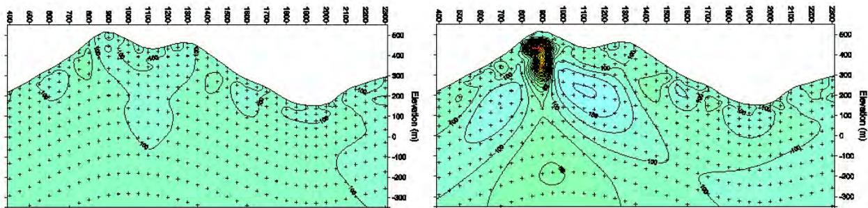
**Figure 7: TE-mode SCS2D 2-D Inversion Model With Topography**
